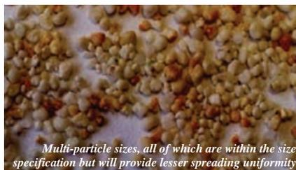
*Multi-particle sizes, all of which are within the size specification but will provide lesser spreading uniformity*
