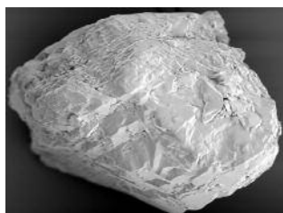
Electron micrograph of sand grain having been treated with Breaker Curative 2
