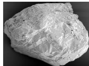
Electron micrograph of sand grain having been treated with Breaker Curative
